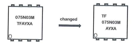
TO-252 series:Product model and printed content, adding "TF" before the original product model;Add the Tuofeng LOGO in the upper left corner of the tube body, the font part remains unchanged, as shown in the following example:
